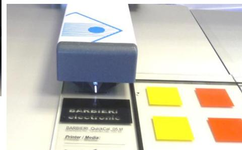
and then continue spot measurement on the patch to be measured:
