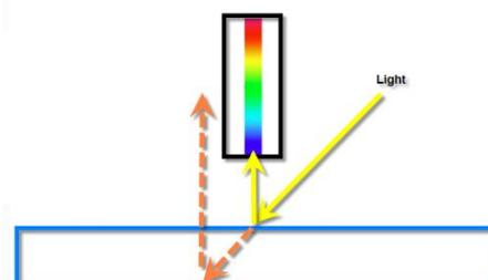
If the printed side is behind the glass, towards the diffuser, reflection measurement is not possible. The reason is, that the light is not reflected back into the optics.
