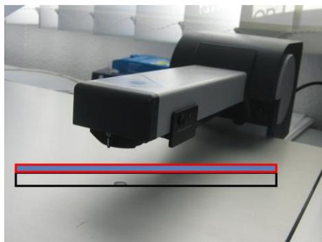
*Print side behind (towards diffusor):* the thicker the glass, the more light can come sideways into the measuring head causing erroneously dark patches to become lighter.
