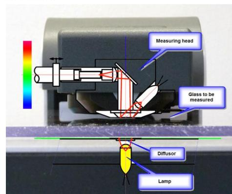
The measuring head touches the glass and is in a distance of the glass thickness to the lamp/ diffuser. In this situation, the measuring head can see also light coming from outside and therefore cause wrong readings. This error does affect only dark colors.
