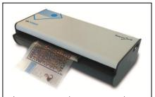
automatic spectrophotometer measuring backlit paper
