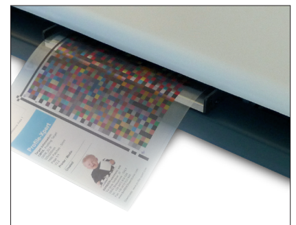
For transparent media to apply color management where images are illuminated from behind
