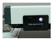
The small aperture corresponds to 2mm aperture, the wide aperture to 8mm.
