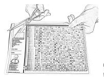
Cut off the reference area of the target to allow the instrument to calibrate to absolute white.
