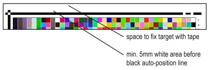
Please verify when inserting the target into the sample holder (specially in transmission), that the space before the auto-position line is visible and not covered by the sample holder or tape.
