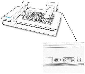
from left to right: on/off switch, power connector, serial port, USB port
