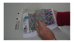
For measuring insert the sample between the two transparent sheets of the sample holder and position inside the corner marks.
